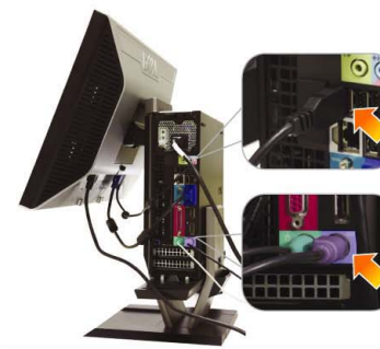
7 Connect the USB, keyboard and mouse cables to the computer as shown
